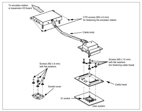
Figure 1 HS36049ECH61H User System Interface Cable
